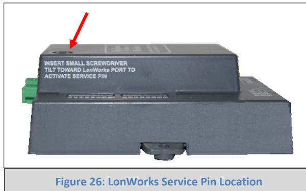
Figure 26: LonWorks Service Pin Location
